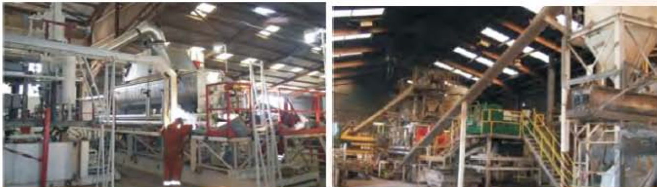
Porcupine Model: Capable of processing 2000 metric tonnes of OBMC per month
